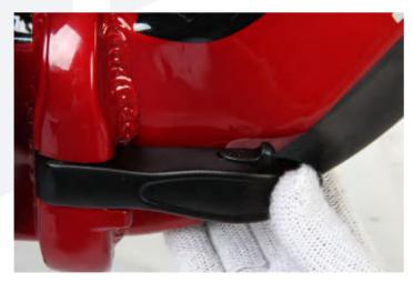
Handlebars: Handlebars can be folded and height adjusted for transport/storage as per initial setup instructions, using the two quick release levers. Ensure levers are secure and safety catches are in place before use.
