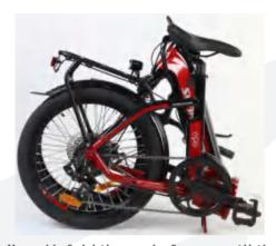
Unfolding: Unfold the main frame until the hinge joint is fully closed and lock it by pushing alloy lock lever until it clamps against the frame. Ensure the Saftey catch clicks into position and the lever cannot open.
