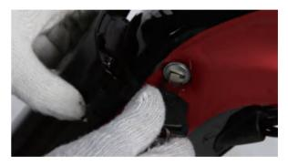
Before loading the battery, please make sure the key lock is in unlocked position. To secure the battery, please turn the key fully anticlockwise after loading the battery.
